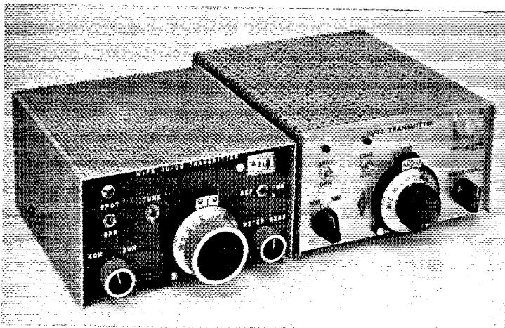
Two versions of the 7- and 14-MHz cw transmitter are shown here. At the left is the W1FB prototype. On the right is a model built by WA6UZO. Both units are small and lightweight.
